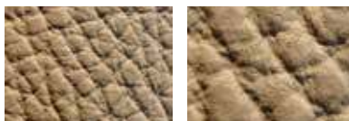
Pigmented smooth leather: the pores are no longer recognizable, a thick layer of dye has been applied to the leather.
