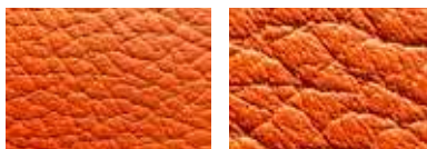
Semi-aniline leather: the pores are clearly visible, but a thin layer of dye has been applied to the leather.
